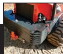
Counterweight bracket 7008601 Counterweight 29 kg 7008285
