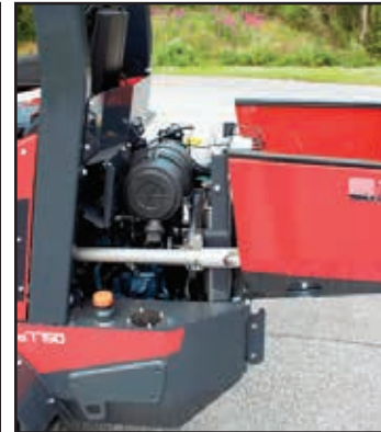
Good access to service and daily maintenance. Lockable engine hood.
