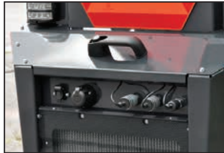
Easy operation of the rear hydraulic outlets. As option 7-p trailer outlet and 3-p control outlet for operating electric valves*.
