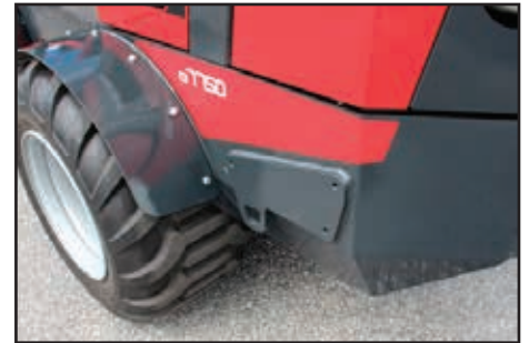
Mounting plate with loop to safely fix the loader for transport. 3xM12 on plate to mount accessories.
