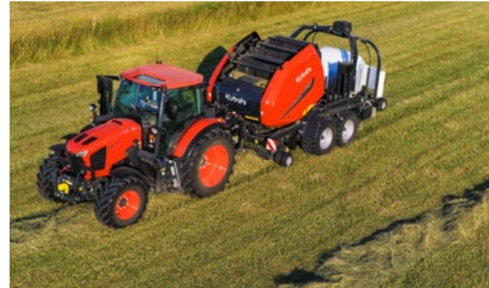
The proven, AEF-certified 7" K-Monitor is available as an option for the M6002. ISOBUS capability and an optional automatic steering system make the tractor ready for precision farming, enabling precise use of resources and efficient headland management.
